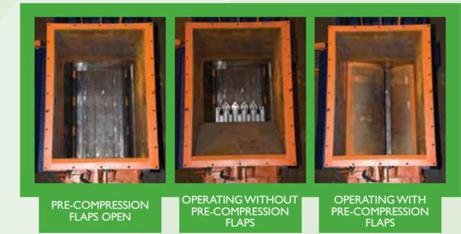
PRE-COMPRESSION FLAPS OPEN    OPERATING WITHOUT PRE-COMPRESSION FLAPS    OPERATING WITH PRE-COMPRESSION FLAPS
